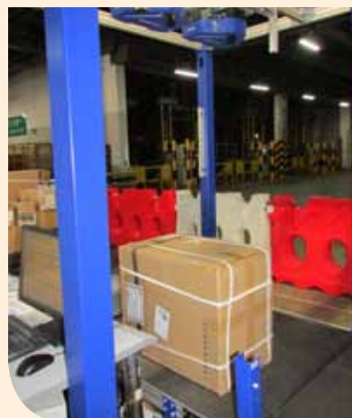
ADS can measure the exact dimension and weight cargo at piece level. 系統能準確偵測及儲存貨物的尺寸及重量。
