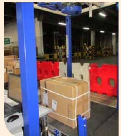
ADS can measure the exact dimension and weight cargo at piece level. 系統能準確偵測及儲存貨物的尺寸及重量。
